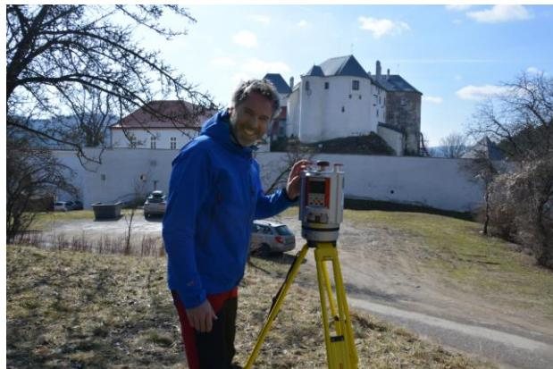
Matej Masný tests LiDAR technology using a terrestrial laser scanner (TLS) at Ľupča Castle
